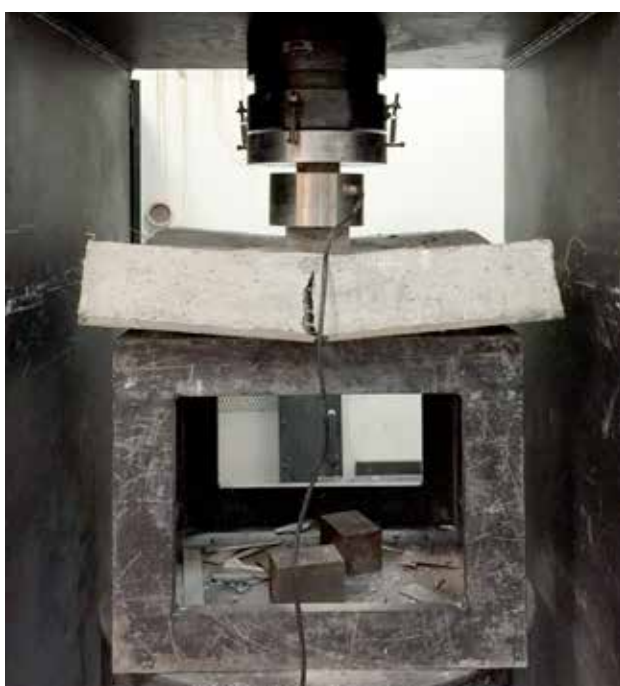
SikaFibre® Force-60 testing according to EN standard.
